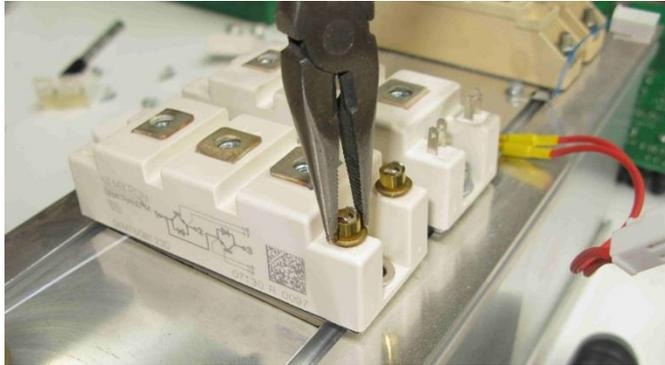
Figure 10-18 25A IGBT stack – remove the gate / emitter shorting rings from new IGBT
