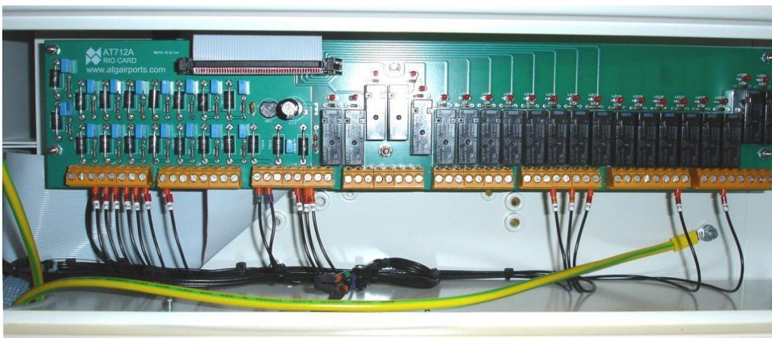
Figure 3-2 AT712 Relay I/O Card fitted in Control Terminal Box
