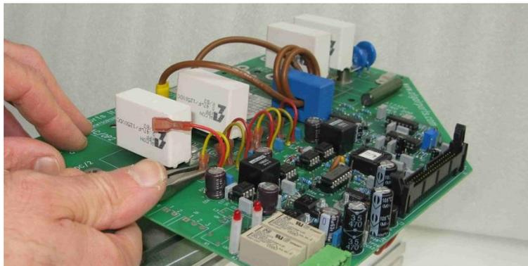
Figure 10-24 25A IGBT stack – re-connection of IGBT gate and emitter driver cables
