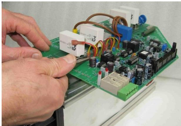
Figure 10-10 25A IGBT stack – disconnection of gate drive cables
