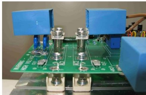
Figure 10-22 25A IGBT stack – Epcos capacitors fitted over diodes
