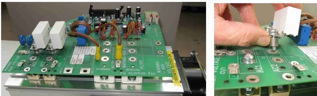
Figure 10-11 25A IGBT stack removal of snubber capacitors and AT732 fixing screws
