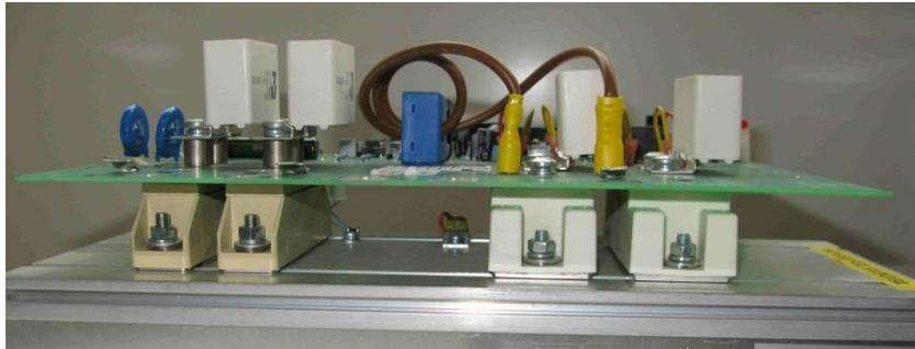
Figure 10-21 25A IGBT stack – re-fit the snubber capacitors
