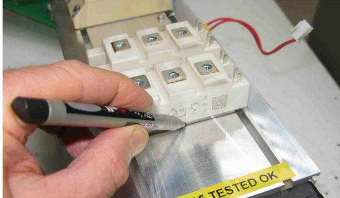
Figure 10-15 25A IGBT stack – mark position of module that is to be removed
