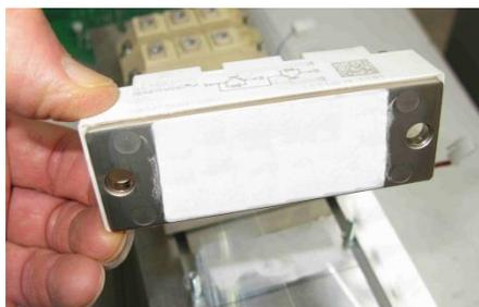
Figure 10-17 25A IGBT stack – smear the back of the module with heatsink compound
