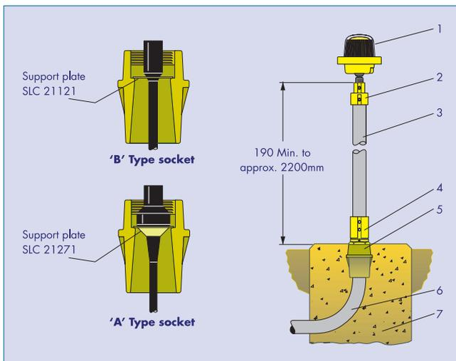
Alternative support arrangements for 'A' or 'B' type socket leads mounted in a wells coupling
