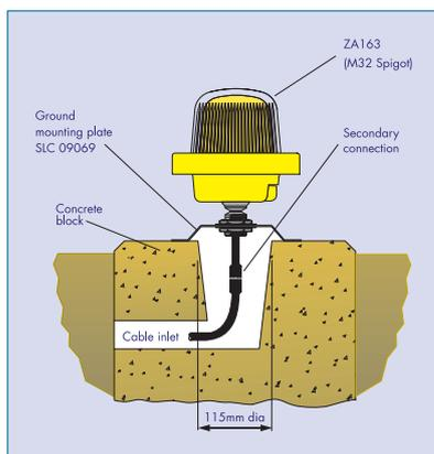
**Note** The ground mounting plate is designed to be held down by means of three 10mm (3/8") rag bolts grouted into the concrete block on 178mm PCD
