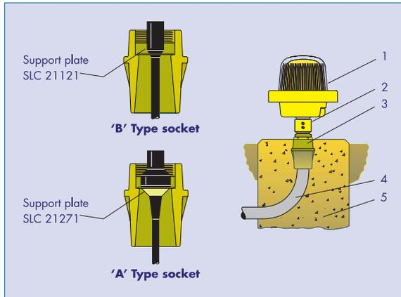
Alternative support arrangements for 'A' or 'B' type socket leads mounted in a wells coupling
