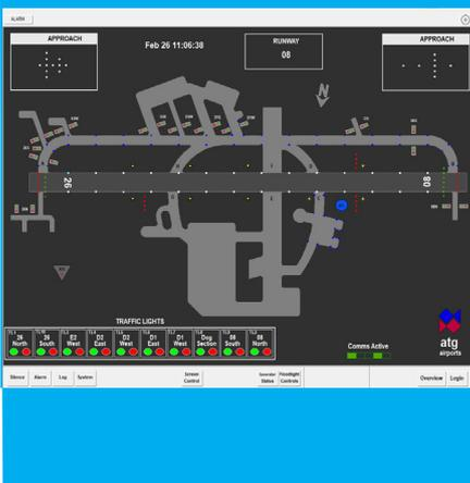
Taxiway circuits on military airfields were generally powered by a Transformer Mains Supply electronic (TMSe) which only has capability to provide 2 stages of brilliancy. Subsequently the TMSe units were replaced with Micro200 Constant Current Regulators (CCR's), and the MCS modified to control and monitor the individual regulators. Again, additional hardware was configured which will enable new taxiways circuits to be connected when they come into service.
